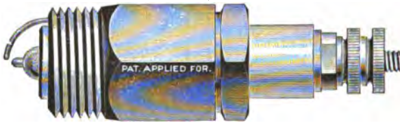
FIG. 331.—"American" Indestructible Sparking Plug. Like the one just shown, this plug has also two essential parts; the shell carrying one electrode, which screws into the metal of the cylinder, and the cone composed of mica, through which runs the other terminal, the two being joined together by screw connections as shown. The superior advantages of mica insulation, as claimed by the manufacturers, are that heat has no effect whatever upon it; thus rendering it much more durable than a plug made of porcelain or other substance liable to be affected by heat and allow short-circuiting of the sparking current.
